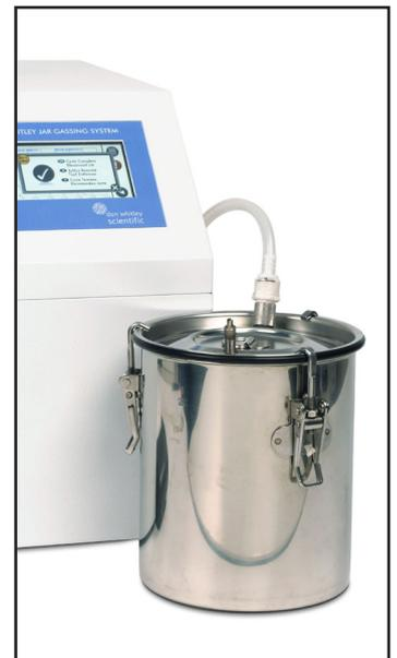
Being constructed from stainless steel, Whitley Jars have other advantages, such as protecting your plates during transport or for growing Thermophiles where the jars need to be incubated at a high heat. They are also fully autoclavable.
